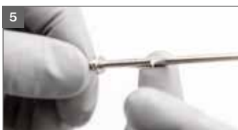
5 Grease paint needle around the needle packing area
