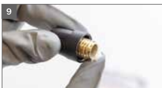
9 Grease thread of material flow control screw
