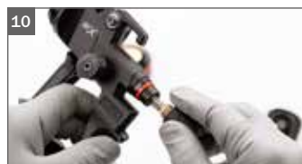
10 Installing material flow regulation screw
